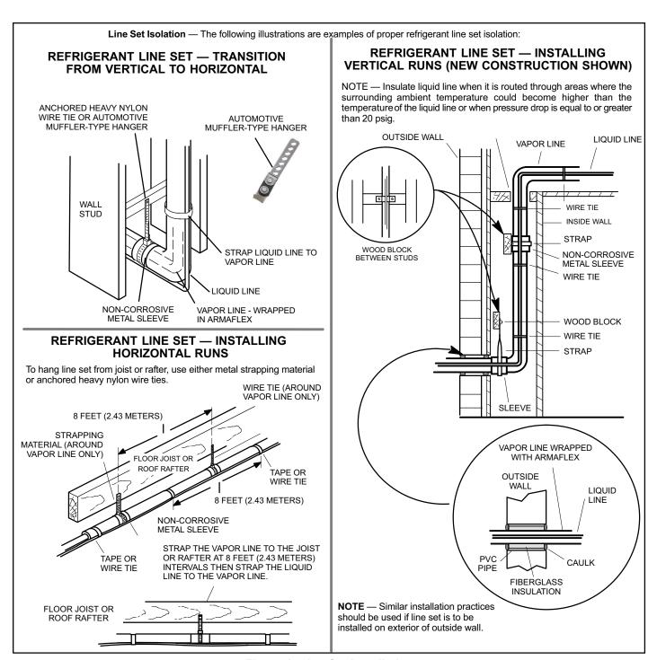
Figure 8. Line Set Installation
